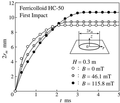
Fig. 4. Evolution of magnetic fluid spread during the first drop impact.
