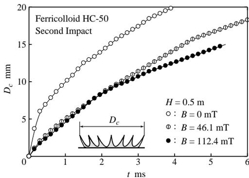
Fig. 5. Growth of magnetic fluid crown edge during spreading at the second drop impact.
