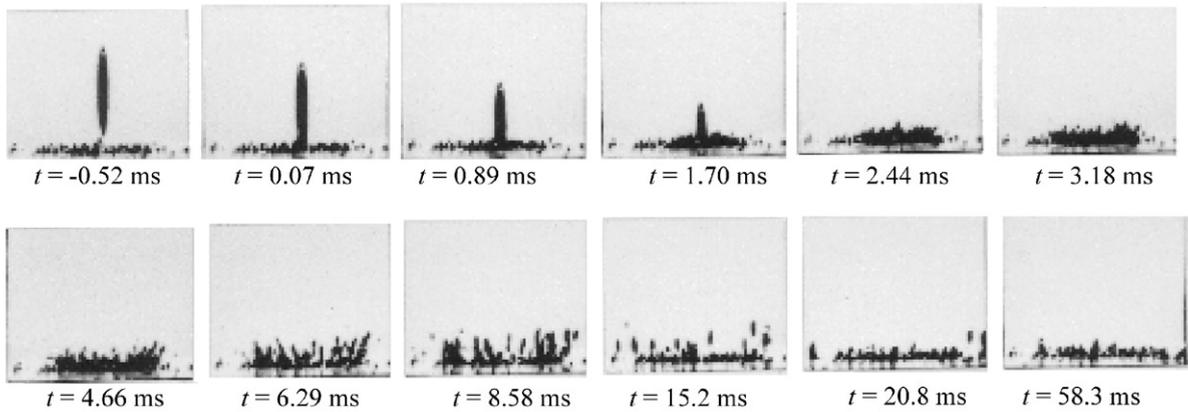
Fig. 3. Photographs of a sequence of stages in the second drop impact with a magnetic field.
