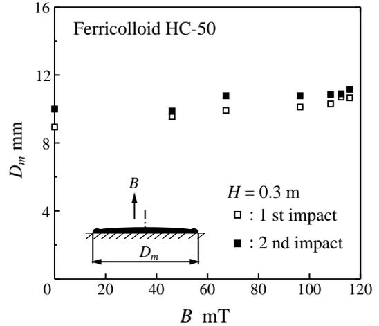
Fig. 6. Maximum diameter of the magnetic fluid spread formed by the drop impact.
