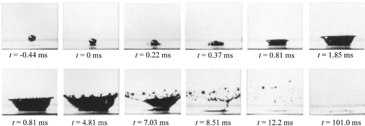
Fig. 2. Photographs of a sequence of stages in the second drop impact without a magnetic field.
