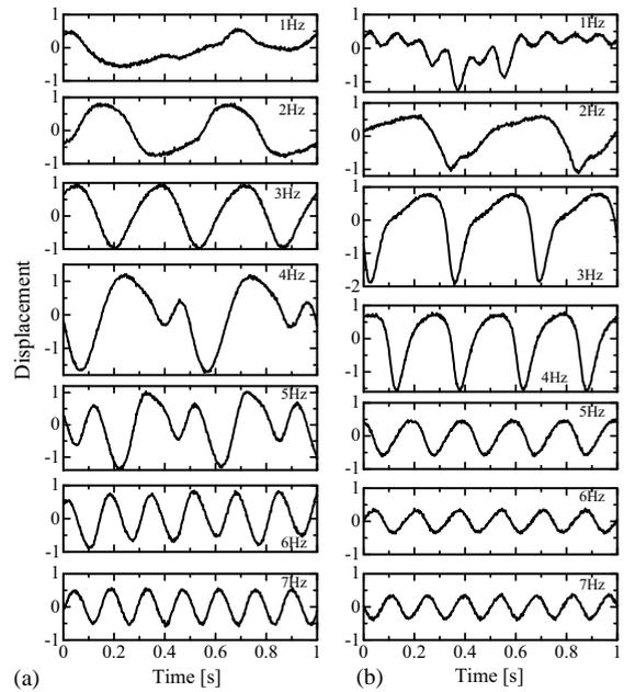
Fig. 3. Displacement of the elastic membrane at the central point of the fluid transportation mechanism. The displacement is normalized by the maximum value (1.67 mm) under the rectangular pulse of frequency 3 Hz. The mechanism is driven by (a) the rectangular pulse and (b) PWM method. The duty ratio of PWM cases is 39%. In both cases, the duty ratio is 39%. The applied electric current is 5 A.
