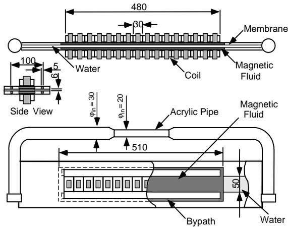
Fig. 1. A schematic diagram of the experimental apparatus of the fluid transportation mechanism.
