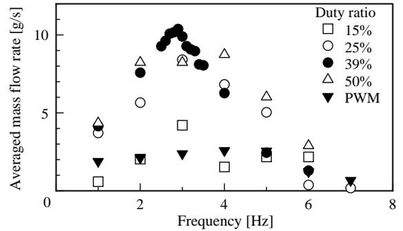
Fig. 2. Averaged mass flow rate changing due to the frequency and the duty ratio. The duty ratio is 39% in the case of PWM. The applied electric current is 5 A.
