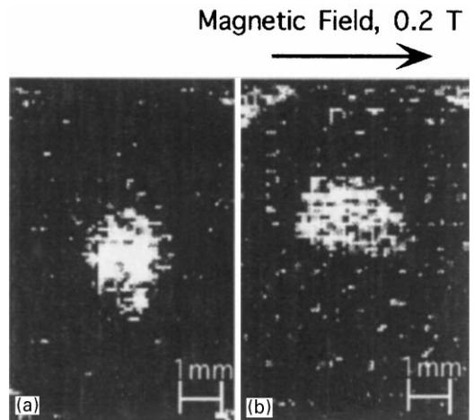
Fig. 3. The analyzed images of air bubble released from a tube from the bottom of the cell, at a constant rate under applied magnetic field strengths of (a) 0, and (b) 0.2 T in water-based MF of 51.2 wt%.
