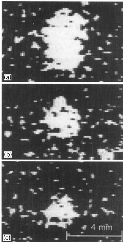
Fig. 4. The analyzed images of air bubble released from a tube from the bottom of the cell, at a constant rate under applied magnetic field strengths of (a) 0, (b) 0.075 T and (c) 0.15 T in ionic MF of 22.7%.
