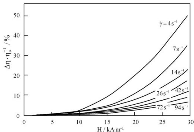
**Figure 10.** The magnetoviscous effect in a commercial magnetite based ferrofluid for various shear rates.
