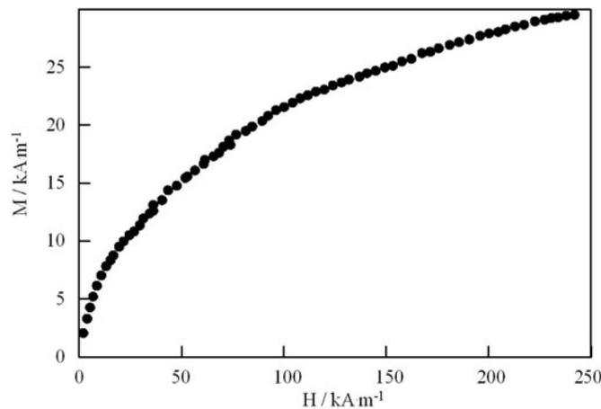
Figure 2. Typical magnetization curve of a ferrofluid.
