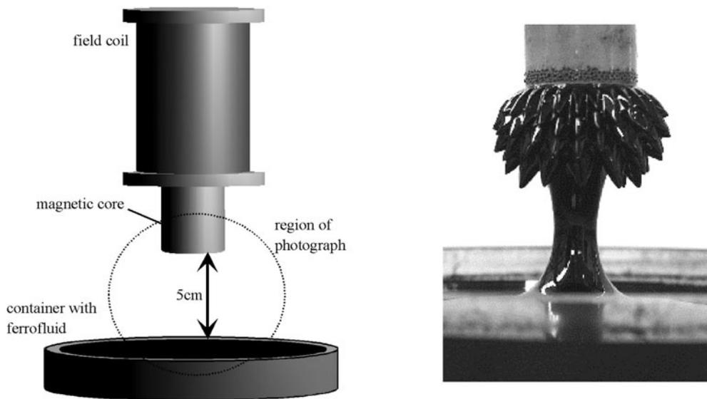
**Figure 3.** The magnetic force exerted by the electromagnet on the ferrofluid in the pool is strong enough to lift the fluid against the earth's gravitational field and to form the characteristic spike pattern.
