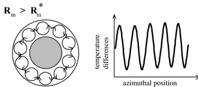
**Figure 7.** The detection of thermal flow of magnetic fluids can be maintained by means of the determination of the temperature distribution at a bounding wall. Further explanations are given in the text.
