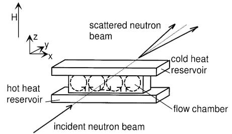
Fig. 1. Sketch of the experimental setup used for the test experiments on flow detection by MSANS.
