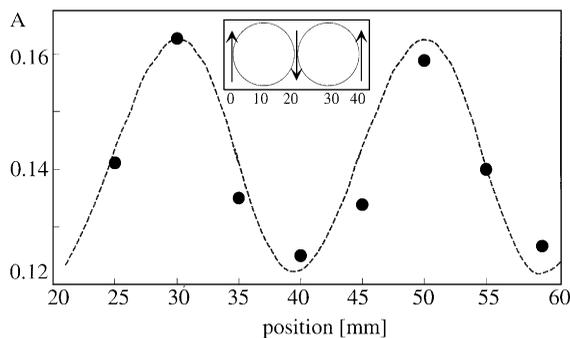
Fig. 3. The anisotropy  $A$  of the scattering pattern corrected by effects due to temperature differences as a function of the position in the  $x$ -direction. The position is counted from one edge of the cell. The inset shows the corresponding flow pattern. The dashed line is a guide to the eye.
