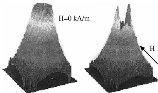
Fig. 2. The measured scattering pattern for  $H = 0$  and 12 kA/m. The axis spanning the base plane corresponds to the positions of the detector cells while the height of depicted surface corresponds to the count rate obtained in the corresponding cell.
