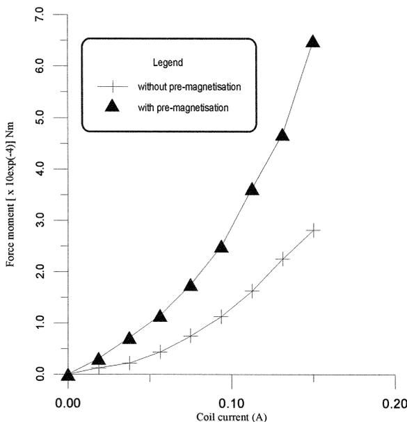
Fig. 2. Force moment vs. current characteristics without and with pre-magnetisation, for  $x_0 = 2$  mm.
