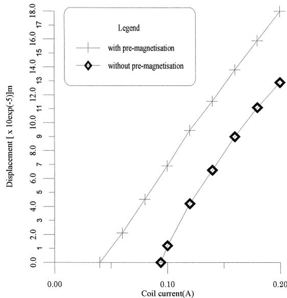
Fig. 5. Displacement vs. current characteristics for the actuator with elastic support ( $x_0 = 2$  mm; the ratio of the displacement transfer,  $r = r_2 / r_1 = 0.5$ ).
