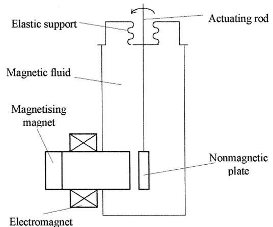
Fig. 4. Actuator with elastic support.
