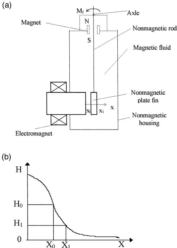
Fig. 1. (a) Actuator with suspension axle. (b) Rate of the magnetic field curve.
