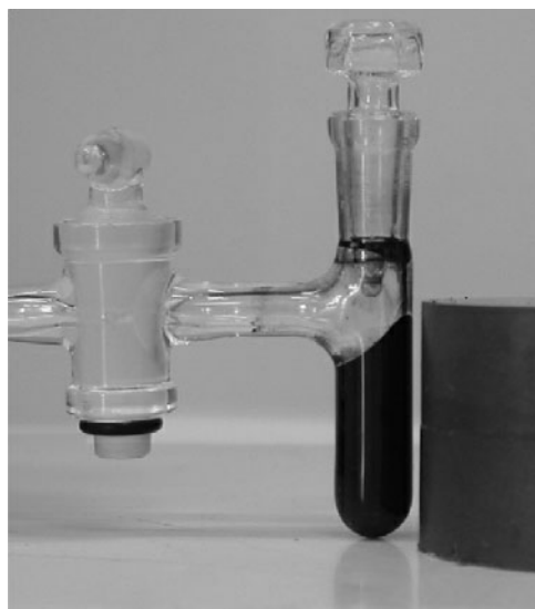
Figure 1. An example of an iron dispersion, synthesized by thermal decomposition of \text{Fe}(\text{CO})_5 in decalin in the presence of modified PIB following [18] and always stored under nitrogen atmosphere. Average particle radii were varied by changing the \text{Fe}(\text{CO})_5 /PIB ratio. The dispersion exhibits the equilibrium shape in a field gradient typical for a stable ferrofluid [16].
