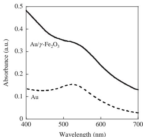
Fig. 1. UV-vis absorption spectra of the aqueous dispersion of (solid line) the present Au/ $\gamma$ -Fe<sub>2</sub>O<sub>3</sub> composite nanoparticles (Au: $\gamma$ -Fe<sub>2</sub>O<sub>3</sub> = 44:56 (wt)) and (dashed line) the monolithic Au nanoparticles.
