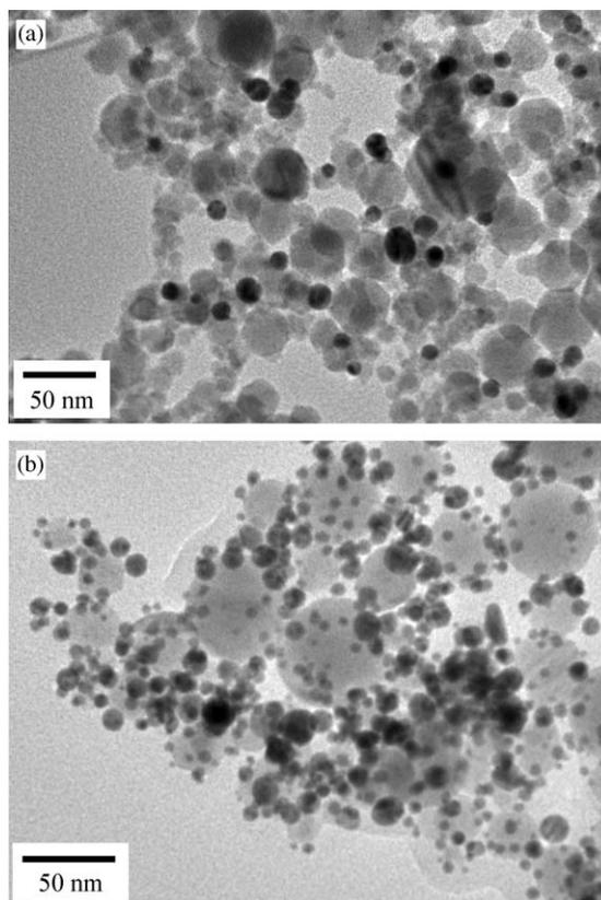
Fig. 2. TEM images of Au/ $\gamma$ -Fe<sub>2</sub>O<sub>3</sub> composite nanoparticles synthesized by gamma-ray irradiation (Au: $\gamma$ -Fe<sub>2</sub>O<sub>3</sub> = (a) 10:90, (b) 44:56 (wt)).
