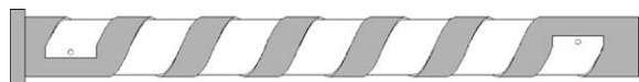
Fig. 2. The helical channel geometry machined into the surface of the polymer cylinder. The original surface of the cylinder is shown in gray with the machined area white in order to highlight the spiral path of the channel. The inlet and outlet ports are shown as small circles at the ends of the channel.
