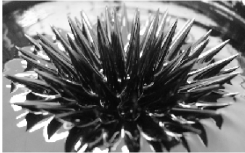
Figure 1: Spiking effect in Kerosene's ferrofluid
