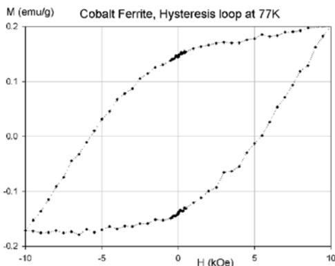
Figure 2: Cobalt ferrite hysteresis loop at 77K.
