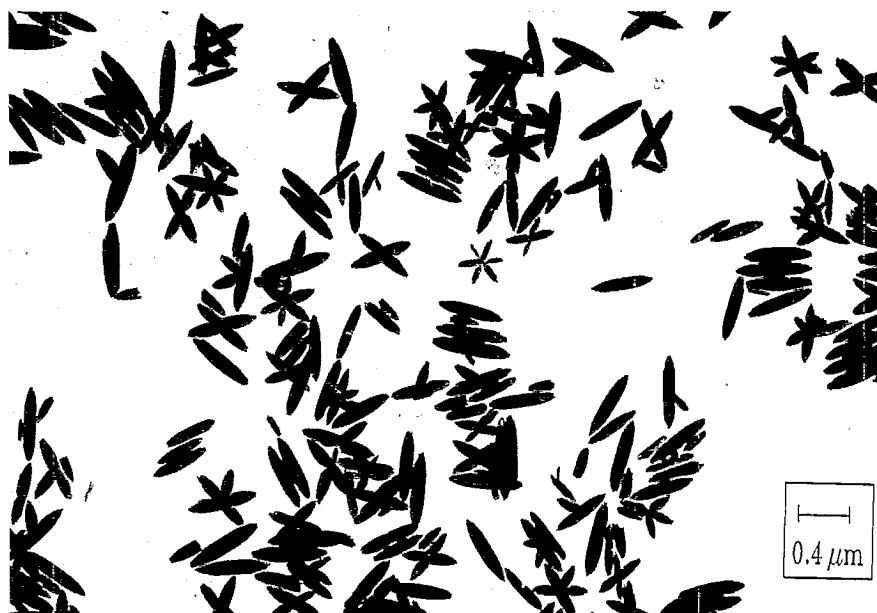
Fig. 3. TEM micrographs of sample S3. Needles, X- and Y-shaped \beta -FeOOH particles are visible.
