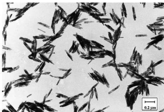
Fig. 5. TEM photograph of \alpha -FeOOH particles of sample G5.
