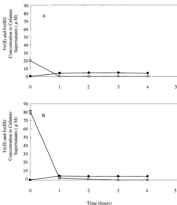
Fig. 3. Fe(III) and Fe(II) concentrations in *M. magneticum* AMB-1 cultures. Early log phase cells were cultured in medium with A: 20  $\mu\text{M}$  and B: 80  $\mu\text{M}$  initial Fe(III) concentration. Fe(II) (●) and Fe(III) (○) were measured using the ferrozine method at different times within the initial 4 h of the cultures.
