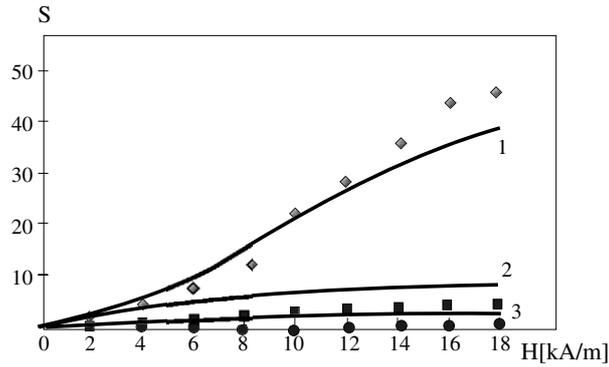
**Figure 2.** The reduced magnetic effective viscosity versus dimensional field  $H$  inside the sample for the magnetite ferrofluid TTR (after [10]). Dots are experiments; lines are results from the chain model. Diamonds and line 1 correspond to  $\dot{\gamma} = 0.1 \text{ s}^{-1}$ , squares and 2 to  $\dot{\gamma} = 1 \text{ s}^{-1}$ , circles and 3 to  $\dot{\gamma} = 10 \text{ s}^{-1}$ .
