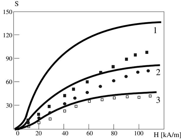
**Figure 4.** Experimental results for the magnetoviscous parameter  $S$  for the monodisperse ferrofluid with cobalt particles 11 nm in diameter, magnetic volume concentration 0.0035, hydrodynamical volume concentration  $\varphi = 0.011$ . Dots are experiments [25], lines calculations. Black squares and line 1— $\dot{\gamma} = 1 \text{ s}^{-1}$ , circles and line 2— $\dot{\gamma} = 3 \text{ s}^{-1}$ , light squares and line 3— $\dot{\gamma} = 10 \text{ s}^{-1}$ .
