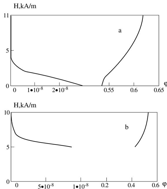
**Figure 3.** Phase diagrams of the magnetite ferrofluid separation into dense and dilute phases for room temperature. (a) The particle diameter is 18 nm, thickness of the surface shell is 2.5 nm; therefore,  $\varepsilon = 7.76$ . (b) The same for the particle diameter 17 nm,  $\varepsilon = 6.3$ .
