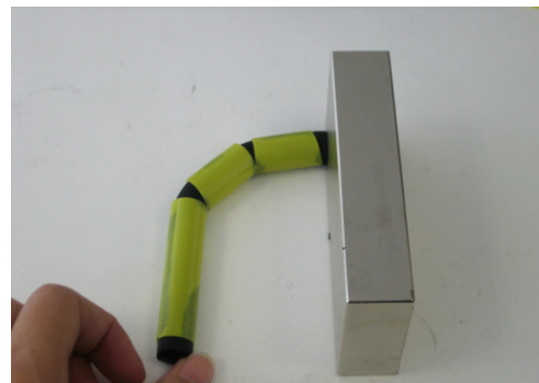
Figure 7. Concentration graded ferrogel, the concentrations are 25, 15 and 3 wt% of iron oxide in the three regions; the highest concentration is closest to the magnet.
