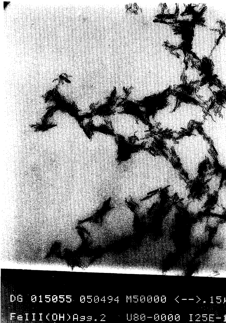
Fig. 4. Cluster of IS particles grown with a lower growth rate as the clusters of Fig. 3. The influence of the reaction kinetic can be seen: the regions of parallel arrangement of the rod-like single particles are larger, resulting in a more dense structure than in the case of fast aggregation.
