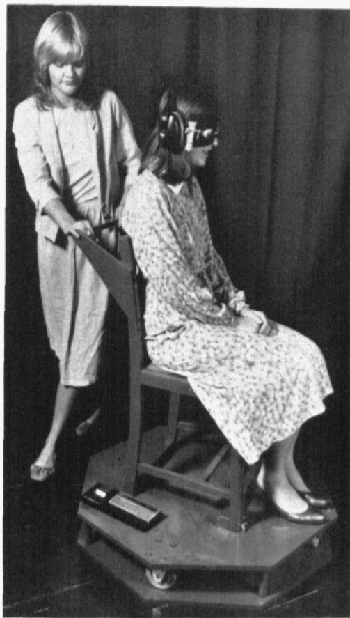
Figure 1 The rotating chair used in the Manchester 'chair' experiments. The pocket computer shown on the base of the chair is normally carried by the experimenter throughout the experiment. This selects and prints out a sequence of random directions, prints out the subject's estimates, and analyses the results (photo by Les Lockey)
