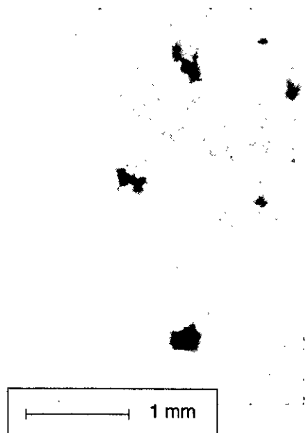
Figure 6. Microfilaments observed with near-normal illumination (pattern centre to the right, main reflection to the left).
